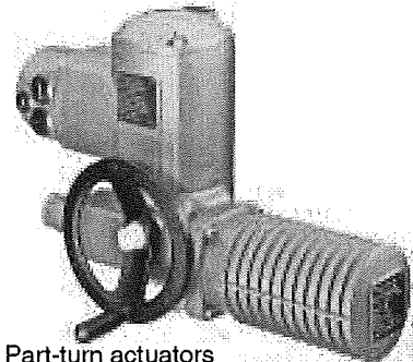
Part-turn actuators SG 05.1 - SG 12.1 Torques from 100 to 1 200 Nm Operating times for 90° from 4 to 180 s
