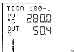
Fig. 3-4 Output OUT is indicated z-19020
