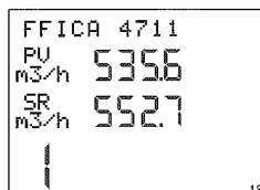
Fig. 3-7 Process value PV= flow A and SP = setpoint flow A z-19019
