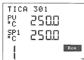
Fig. 3-38 Remote control is active z-19035
