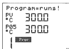
Fig. 3-19 During running program switching z19016 to other setpoints is not possible
