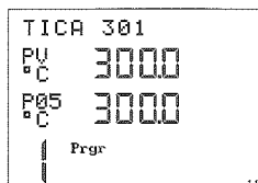
Fig. 3-15 Programmer has stopped. z-19011 Program (Prgr) is flashing.
