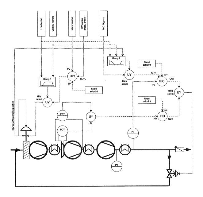
PIC pressure controller power controller UIC surge controller FIC =
