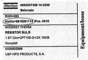
Parts label with detailed information about delivered parts it is possible, that the part no. is the same number as the drawing no.
