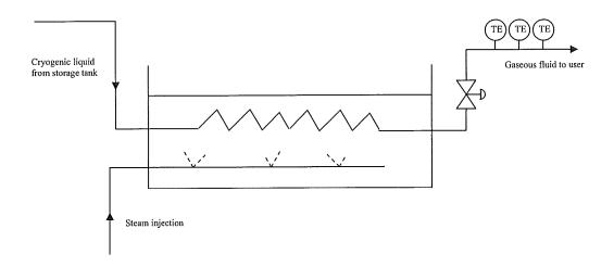
Black up systems installed to provide a high reliability of gaseous products supply ensure the vaporization of the cryogenic liquid by a heat exchange with hot water. Since the some piping and equipment cannot withstand cold temperatures, the verification that the completed vaporization of the liquid and that the heating of the gas up to ambient temperature are performed is essential.
